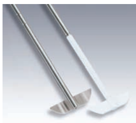
USP 2 UniShaft® in st. steel and Teflon finish; PEEK paddle
