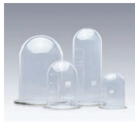
Vessel sizes: 250 ml, 1000 ml, 2000 ml and 4000 ml
