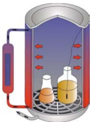
The Laboklav 55 -195 series' recooling system operates according to the heat exchanger principle. Demineralized water from the storage tank passes through the double jacket, cools the entire chamber and flows back into the storage tank where it is cooled down by a cooling coil fed with tap water.
