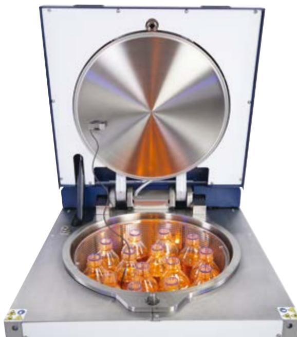
Steam exhaust condensation is integrated as standard into all units to protect the drain pipes. Any condensation forming is cooled by the addition of tap water at the outlet and your drain pipes are thus protected from damage by steam and hot condensate. A PT100 temperature sensor controls the temperature at the unit's outlet and regulates the addition of tap water. The temperature at the outlet can be gradually adjusted.
