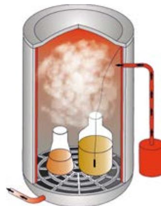
Steam generation using the built-in steam generator
