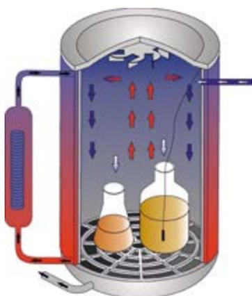
The combination of a water recooling system with counter pressure and a built-in fan is the fastest and most effective recooling system. The powerful fan mixes the temperature gradients in the chamber during the cooling process and ensures uniform and quicker recooling.
