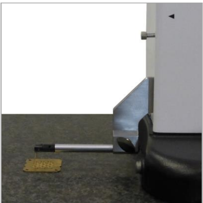
Height measurements on watch movement plate
