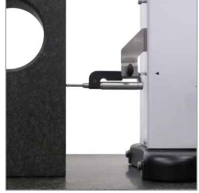
Perpendicularity measurements with electronic probe
