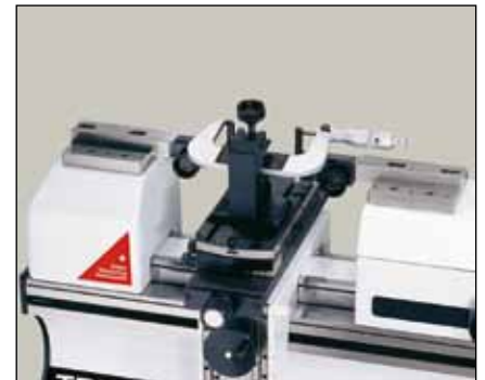
Calibration of external micrometers (HPA-1/TULM14)
