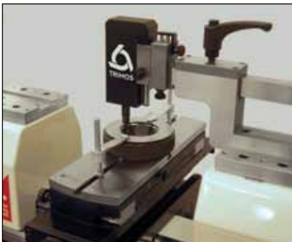
Calibration of thread ring gauges (TA-SU-313/LABC-70/TA-SU-354)
