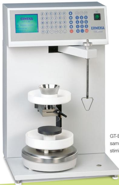
GT-B for automatic determination of the sample repose angle\* and with optional stirring device\*.
