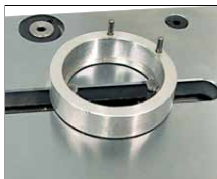
Checking of internal grooves (TELS10)
