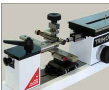
Calibration of plain and threaded plug gauges using the floating table (THV-115)
