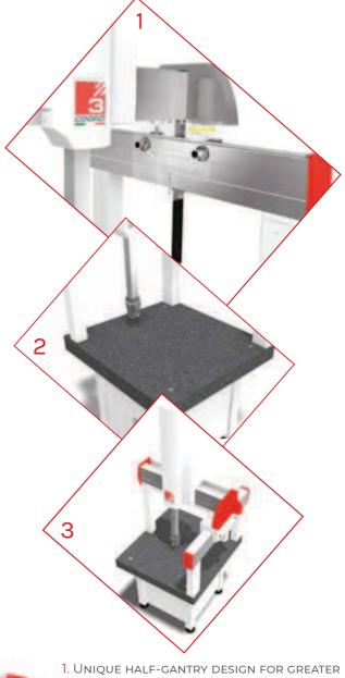
Unique half-gantry design for greater rigidity and lower inertial mass
