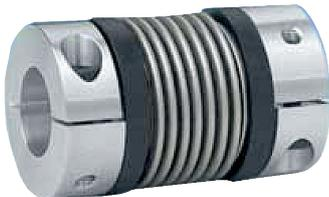
For optimum compensation of misalignment we recommend torsionally free metal bellow couplings. They are characterized by their excellent torsional stiffness during torque load and their low restoring forces. The couplings are optionally with keyways available. For further information please see accessories data sheet 869X.
