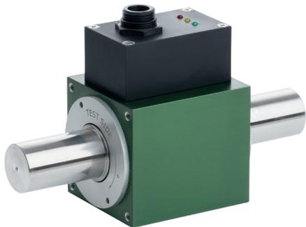
This sensor version has a USB connection instead of the  $\pm 10$  V output. The sensor is powered via USB, no further connections required. In addition to torque, the speed or rotation angle measured values are optionally available. The calculated mechanical performance in is also displayed in DigiVision. Free drivers are available for integration into LabVIEW and DASyLab, also a DLL for integration into your own programs.
