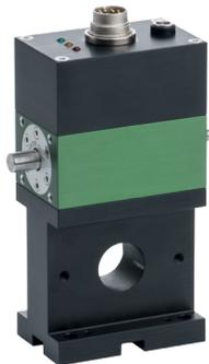
If the sensor needs to be replaced, the locating pin speeds up replacement, avoiding the need for laborious realignment. This can be useful especially when the sensor is only used occasionally in the load path. The mounting block has a central hole and special design allowing a range of options for reliable cable attachment. Two clips ensure the sensor is fixed securely. For further information please see accessories data sheet 8661-Z00X
