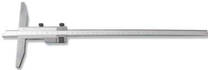
**Depth measuring monoblock caliper** in hardened stainless steel. Satin-chromed readout scale. Etched, precision graduation, easy to read and long-lasting. Raised slider for easy movement. Slider locking screw with micrometric adjustment. Suitable **for modelmakers** having the following etched contraction scales 1% - 1.5% - 2% - mm. Serial number. Manufactured as per DIN 862. Supplied in case.
