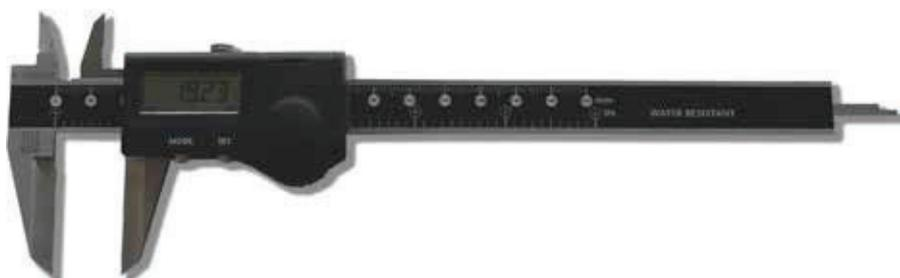
**Digital caliper** in hardened stainless steel. 5 figure liquid crystal display and minus sign. mm/inch conversion. Set to zero in any position. RS232C output to printer port. Slider locking screw. Battery powered. Automatic switch-off. **Knife jaws**. Serial number. Manufactured as per DIN 862. Supplied in case.
