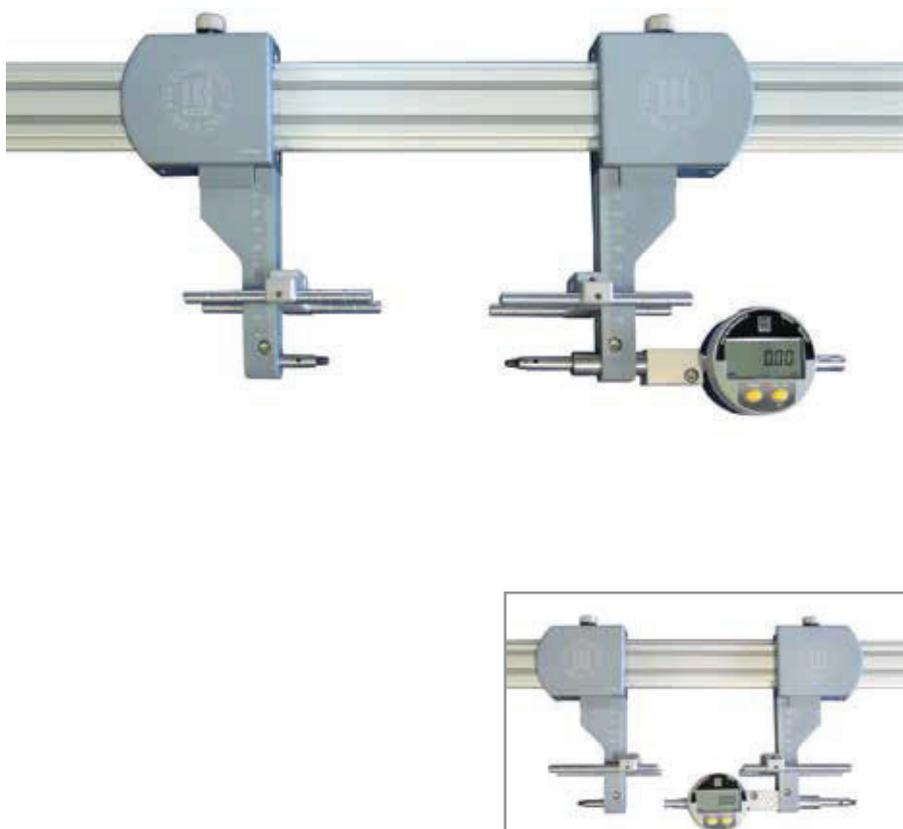
**Rectangular profile 40x20 mm made of special hardened alloy hot that ensures rigidity and lightness. Anodization treatment which makes it scratch-resistant and corrosion-proof, with hardness of 250÷350 HV. Sliding guides made from ø 6 mm steel rods hardened and ground.**
