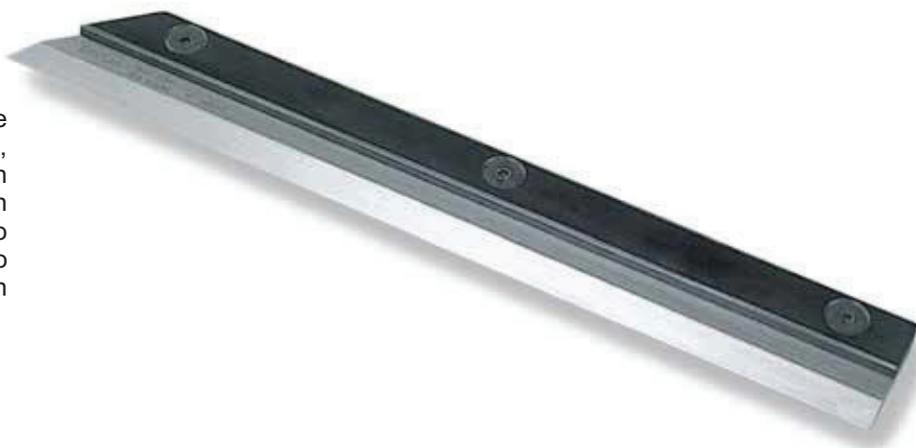
*Hardened stainless steel **knife-edge** straight edge for fast and precise control of planarity and parallelism. Made from hardened stainless steel, ground with lapped contact angle. Fitted with heat-insulated grip. Manufactured as per DIN 874/00. Supplied in case.*
