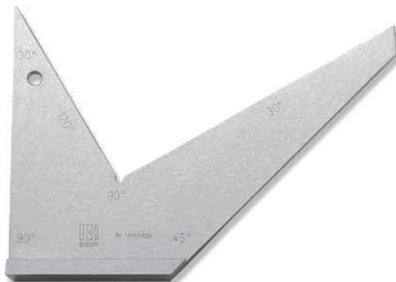
**Onglet square** in non-deformable steel with anti-corrosion treatment. This square has four angles: 90° - 45° - 30° - 120°. Entirely ground surfaces. Manufactured as per DIN 875/2.
