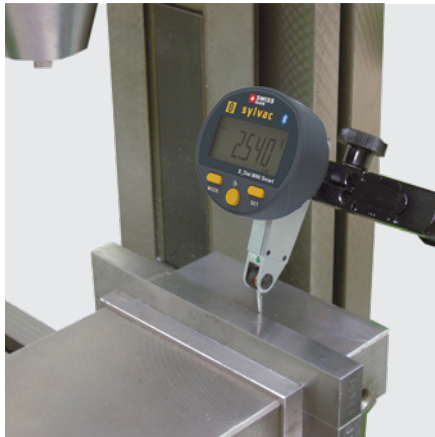
Checking the alignment on milling machine.
