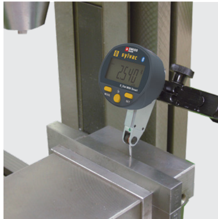
Checking the alignment on milling machine.
