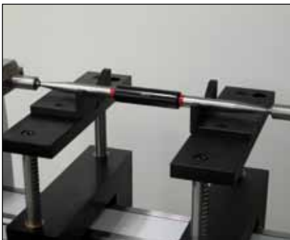
Calibration of gauge bars (TELM7/TELMN7.2)
