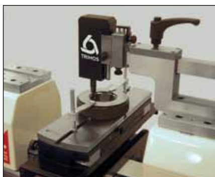
Calibration of thread ring gauges (TA-SU-313/LABC-70/TA-SU-354)
