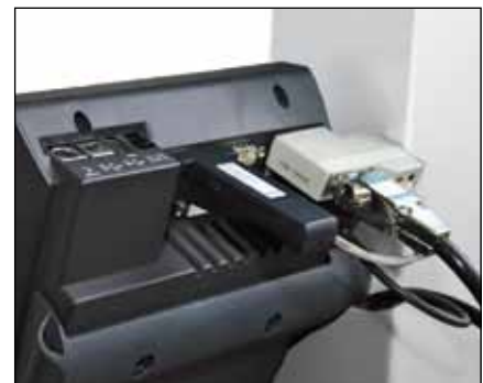
Wireless communication by Bluetooth or Wi-Fi (optional) (TA-EL-123/4)
