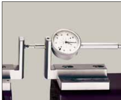
Checking of dial indicators (TEL5CN)
