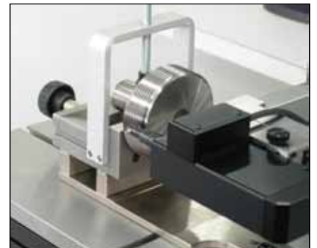
Checking of taper thread plug gauges (TA-MS-381/TEL75)
