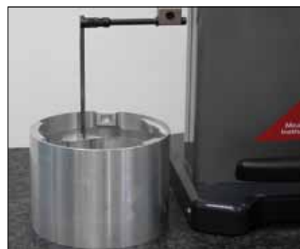
Depth measurement (TA-IH-109/V-50.5/V-50.4)
