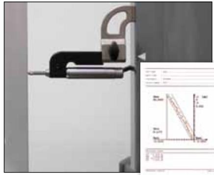
Checking of squareness using an additional electronic probe and colour print-out of the curve (TA-MS-101)
