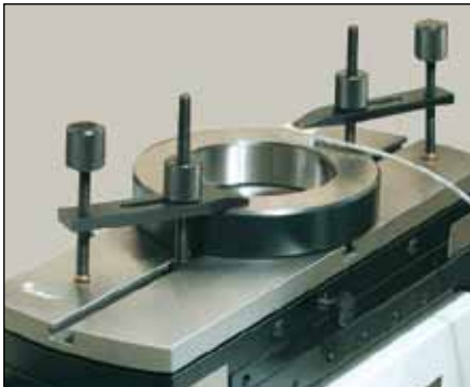
Temperature compensation system TempComp
