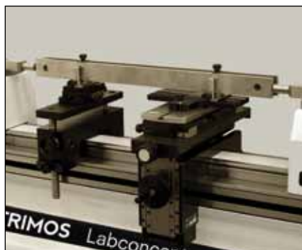
Comparative checking of gauge blocks > 250 mm (TA-SU-313/TELMA7/P/TA-SU-305/TA-SU-306)
