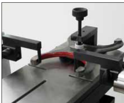
Calibration of snap gauges (TEL16.1/TEL14N)
