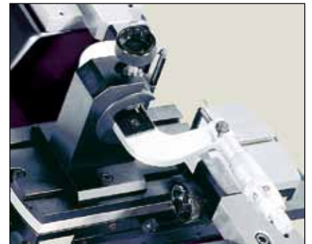
Checking of external micrometers (HPA-1/TULM14)
