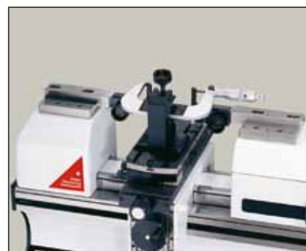
Calibration of external micrometers (HPA-1/TULM14)
