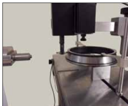
CNC controlled external taper ring measurement
