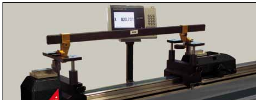
Setting of a large gauge (TEL5)
