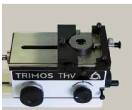
Calibration of plain rings gauges (THV-260)
