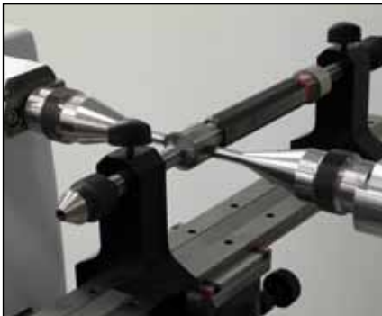
Calibration of plug gauges (TULM6/L05/TA-SU-315)
