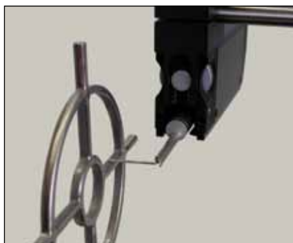
Transversal flank measurement (TA-MS-627)
