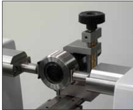
Calibration of thread plug gauges (3P/0.17-3.2/S6.5/TA-SU-315)
