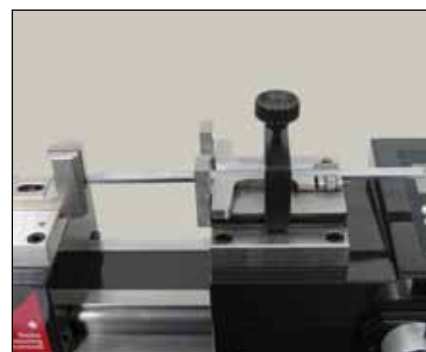
Checking of depth gauges (TULM19/TEL5)
