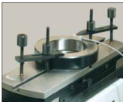
Integrated temperature compensation system TempComp
