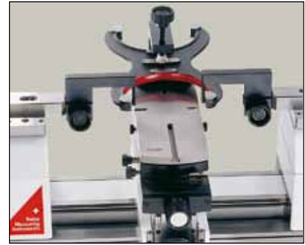
Checking of snap gauges (TA-SU-313/TEL14N)
