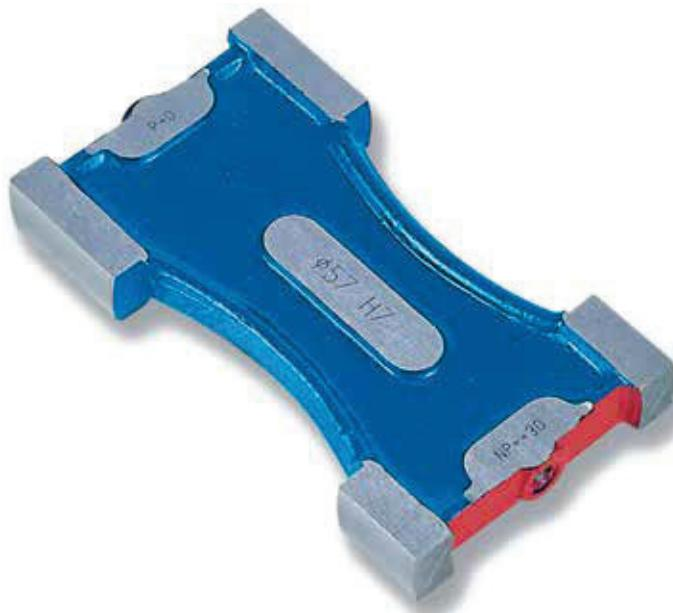
**Flat plug gauges "Go-No Go". Rigid body in stabilized special steel C10. The calibrating sections are case-hardened and tempered hardness >62 HRC. Range Ø 22-103 mm.**
