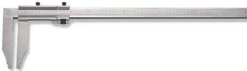
***Monoblock caliper** in hardened stainless steel. Satin-chromed readout scale. Etched, precision graduation, easy to read and long-lasting. Raised slider for easy movement. Slider locking screw with micrometric adjustment and lapped contact surfaces.*
