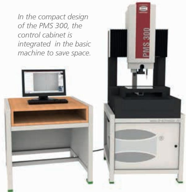
*The base frame, including the measurement tables of the PMS 300-700 series are made entirely of granite. This guarantees the highest levels of stability and reproducible measurement results.*
