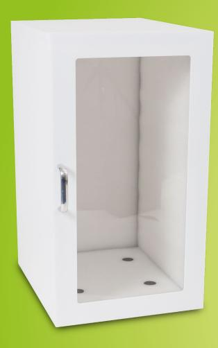
The ERWEKA noise chamber is the perfect companion to our tapped density testers. Crafted from carefree plastic and lined with 30 mm thick, white EPE dampening material, the noise chamber reduces noise of a tapped density tester of approximately 25 db(a) (measured from a standard, horizontal distance of 0.65 m away).
