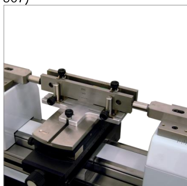
Comparative control of gauge blocks 100 ÷ 250 mm (TA-SU-313, TA-SU-305)
