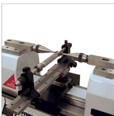
Calibration of threaded plug gauges (HPA-1, TEL6, 3P/0.17-3.2 /S6.5, LABC-15)
