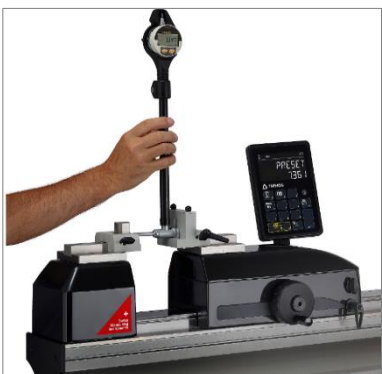
Manually checking of external micrometer (TA-SU-301, TEL5)
