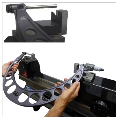
Manually checking of external micrometer (TEL5) (TEL11)
