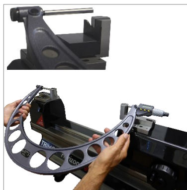
Manually checking of external micrometer (TEL5, TEL11)
