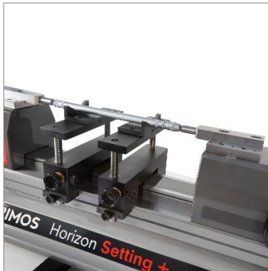
Setting of 2-point internal measuring equipment (TELMA7)
