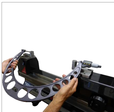
Manually checking of external micrometer (TEL5, TEL 11)
