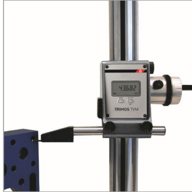
Diameter measurement with bidirectional probe (TVM4)
