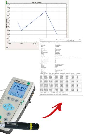
The high-precision calibrator and tester model 7281 is ideal for locating faults in measurement systems. For display devices based on strain gauge sensors, the stored characteristics values can be simulated in an infinitely adjustable range of  $\pm$  3 mV/V and  $\pm$  50 mV/V. In this case it is also important to measure the excitation voltage for strain gauge sensor in order to rule out any problems here.
