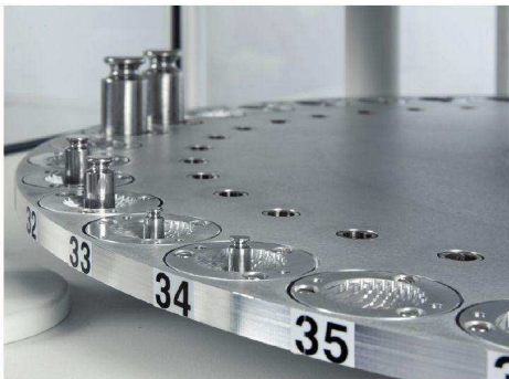
Possibility to load 36 objects onto the comparator's magazine. This allows to calibrate the whole set of weights during one course.
