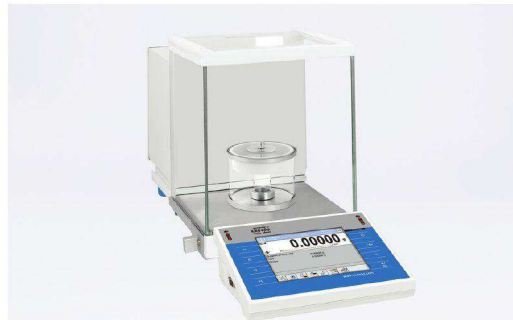
XA 4Y.M.A microbalance with additional adapter for pipettes calibration
