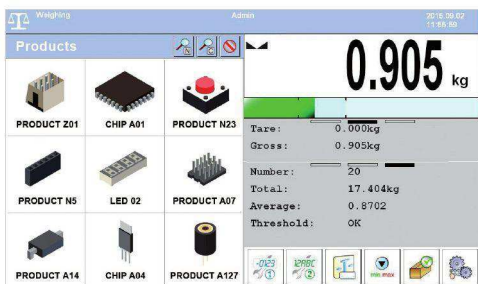
HY 10 terminal features pictograms database providing you with icons that can be assigned to weighed products.
