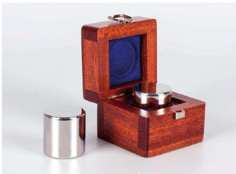
Additional mass standard with magnetic susceptibility determined by NMI enables verification and calibration of the susceptometer.
