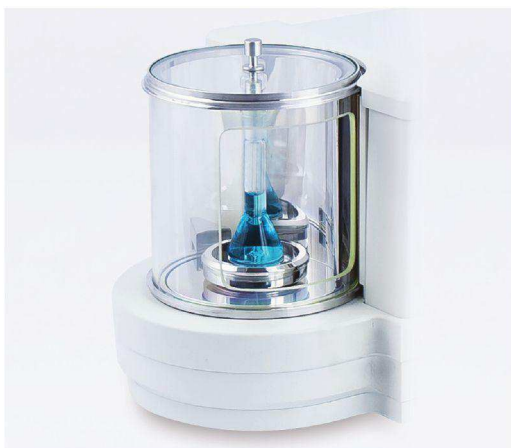
Mass measurement of liquids using MYA 4Y microbalance
