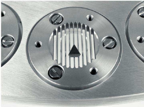
Comparison of very small 1 mg plate mass standards without the threat of jamming.
