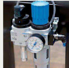
Compressed Air Service Units
