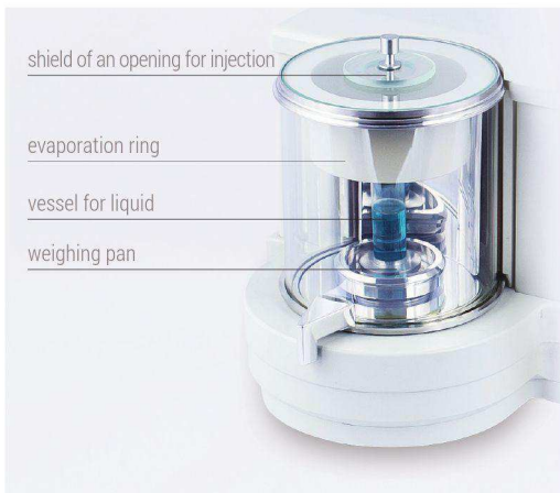
MYA 4Y.P microbalance for pipettes calibration
