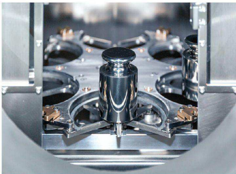
Suspended weighing pan of custom design eliminates eccentricity errors and facilitates dropping the weight onto the magazine insert correctly.
