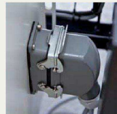
Quick coupling allowing easy detachment of conveyors
