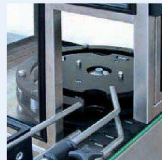
Rotational feeder of cylindrical products
