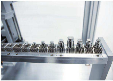
The RMC mass comparator is equipped with 100-position magazine.
