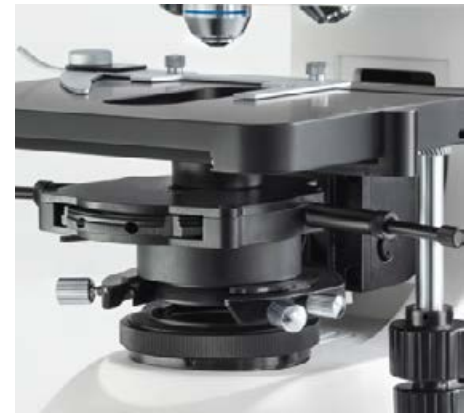
OBN-15: Mounted phase contrast condenser
