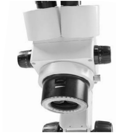
Dimmable, integrated LED ring illumination
