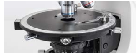
Center-adjustable and turnable polarisation stage
