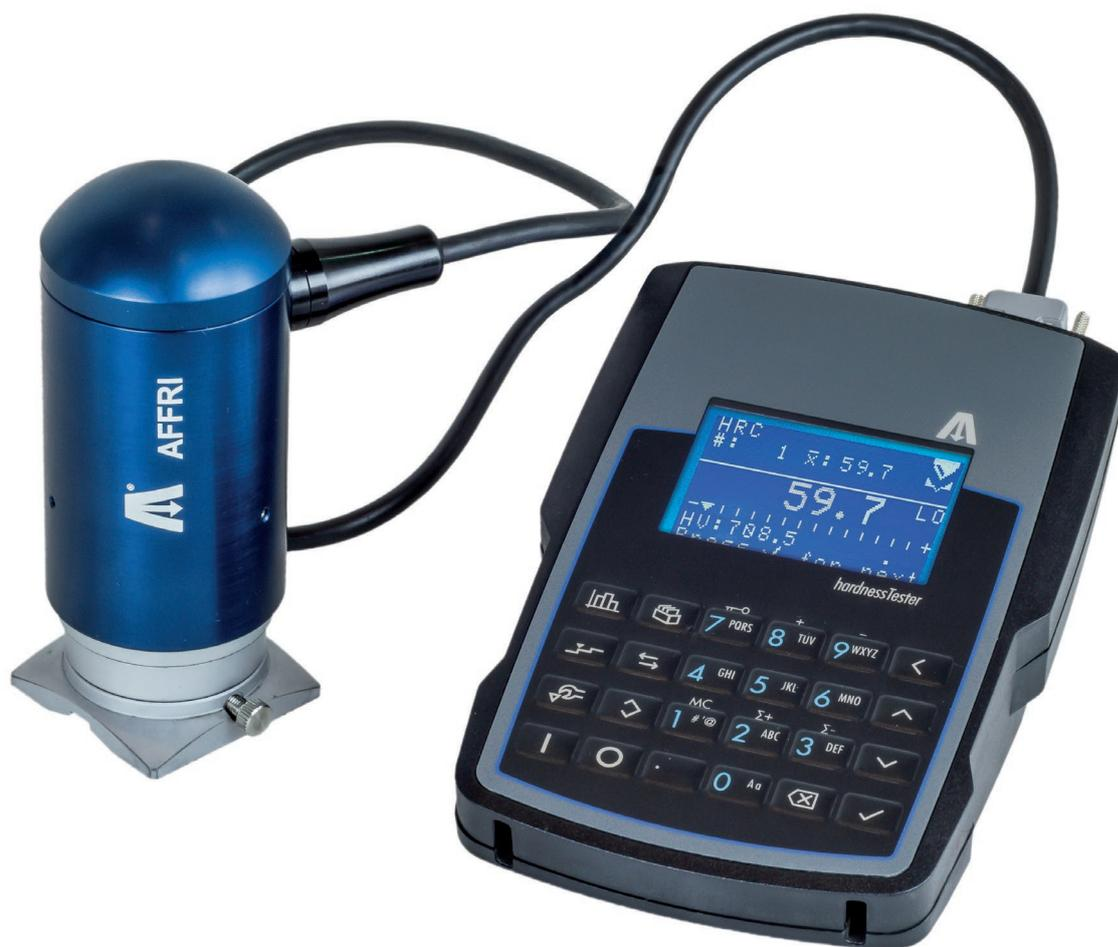
MICROPROCESSOR CONTROLLED DIGITAL DUROMETER
