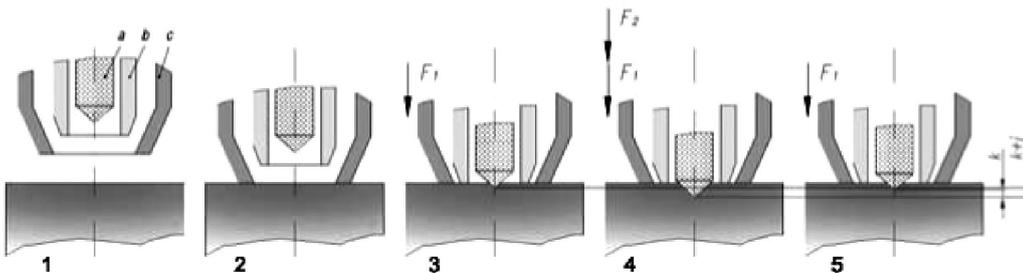
It works neither by rebound nor by means of ultrasounds, it works with a static load and it measures the penetration. It can test hardness of coatings or of foil as thin as 0.08 mm.
