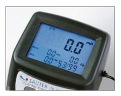
Premium coating thickness gauge for paint coating, lacquer coating etc.
