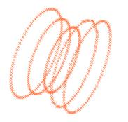
▲ A lot remains questionable Important data can remain hidden between the measurement circles, as actual measurement points are missing.
