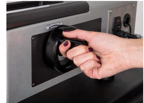
The manual knob allows you to manually control the focus.
