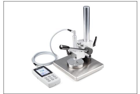
Test stand for repeatable movements during testing. In this way you can avoid errors which could occur in manual handling of the sensor. This ensures even more stable measurements and more precise measuring results, see *accessories*
