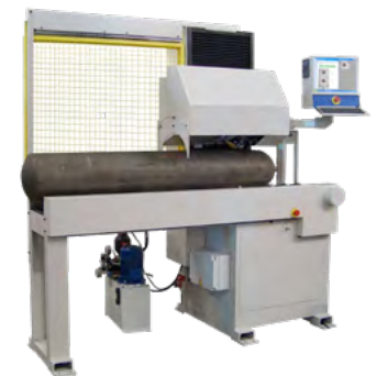
INTEGRAL BOTTLE Brinell up to 3000kgf. Fully automatic multi-indentation cycles on cylinders and bottles. Built-in programmable milling.
