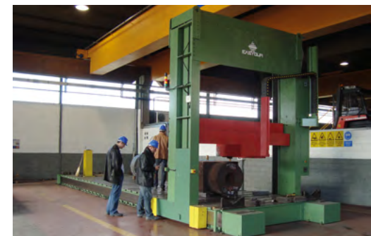
PORTALE CNC portal for Brinell tests up to 3000kgf, 14 m, 4 axes with programmable milling included and automatic test cycle with image analysis.
