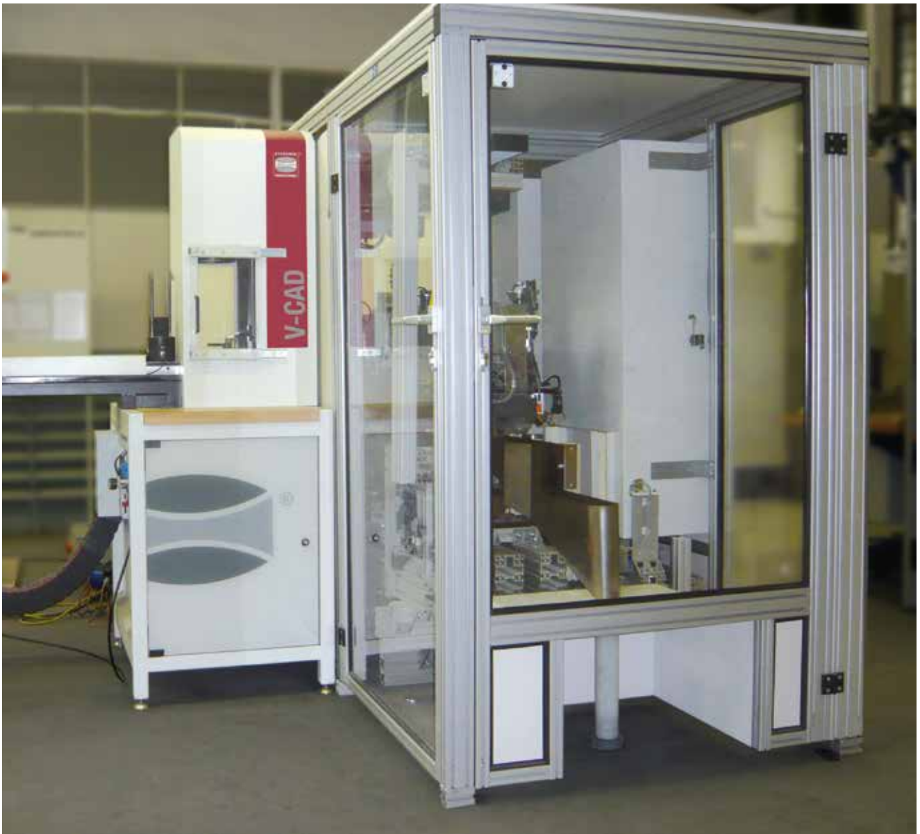
Measuring cell with two V-CAD modules and adjacent packaging unit.
