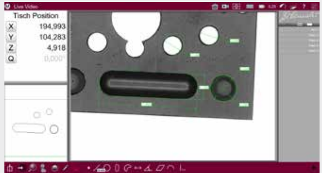
The sector incident light can also be used to accurately record and measure elements on the surface of the workpiece.
