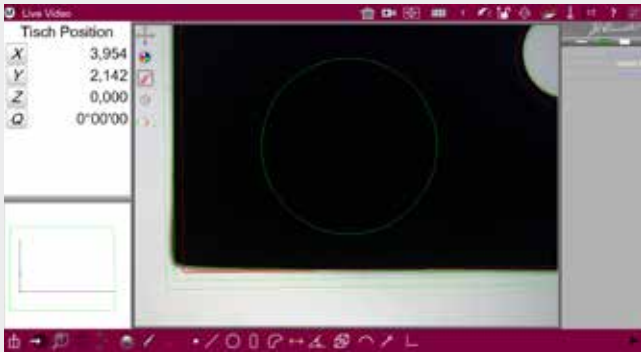
Optical comparison of "good/poor" including tolerance range that can be generated freely to actively support operation.
