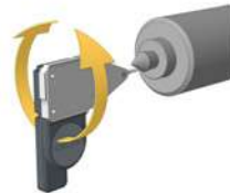
Circular geometry and location measurement on lathe counter-spindle
