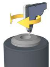
Circular geometry measurement and localization on milling machines
